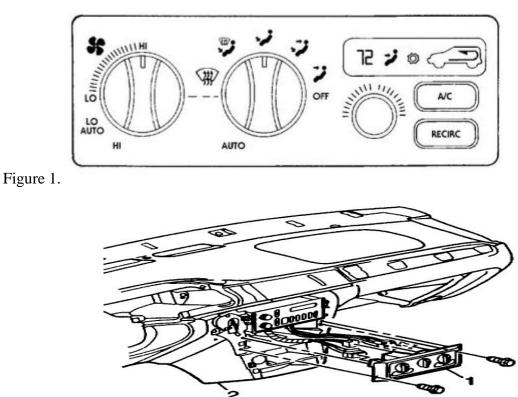
(1) Heater and A/C Control Assembly Figure 2. (2) Instrument Panel
